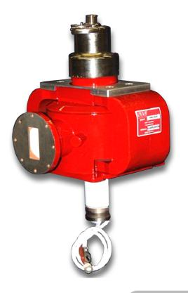
The VMC2033A is a coaxial magnetron that delivers high peak and average RF power for use in weather radar transmitters.
